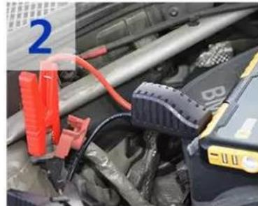
**2** Red clamp on positive (+) terminal, black clamp on negative (-) terminal of battery
