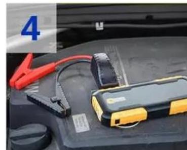
**4** Take the clamps off within 30 Seconds after finishing starting
